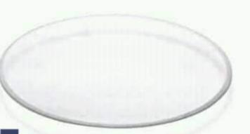
a circular, slightly curved piece of glass used in chemistry as a surface to evaporate a liquid, to hold solids while being weighed, or as a cover for a beaker
