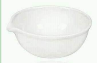
a porcelain or ceramic dish used to used to evaporate excess water (or other solvents) to ensure that a concentrated solution or the dissolved substance is left behind
