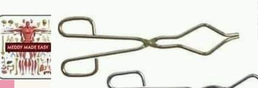
tongs used to carry a crucible after it has been subjected to heat and/or cold temperatures
