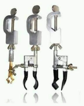
a device (shaped like a "C")used to hold or secure objects to a retort stand.
