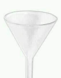
used to channel liquid or finegrained substances into containers with a small opening
