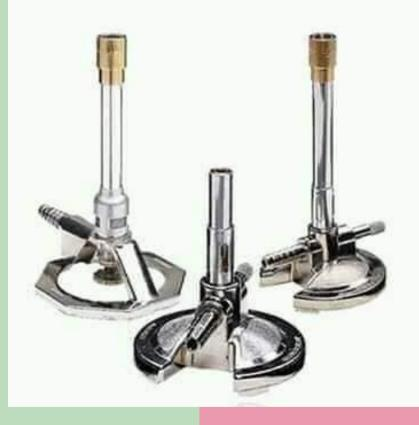
piece of laboratory equipment that produces a single open gas flame, which is used for heating, sterilization, and combustion
